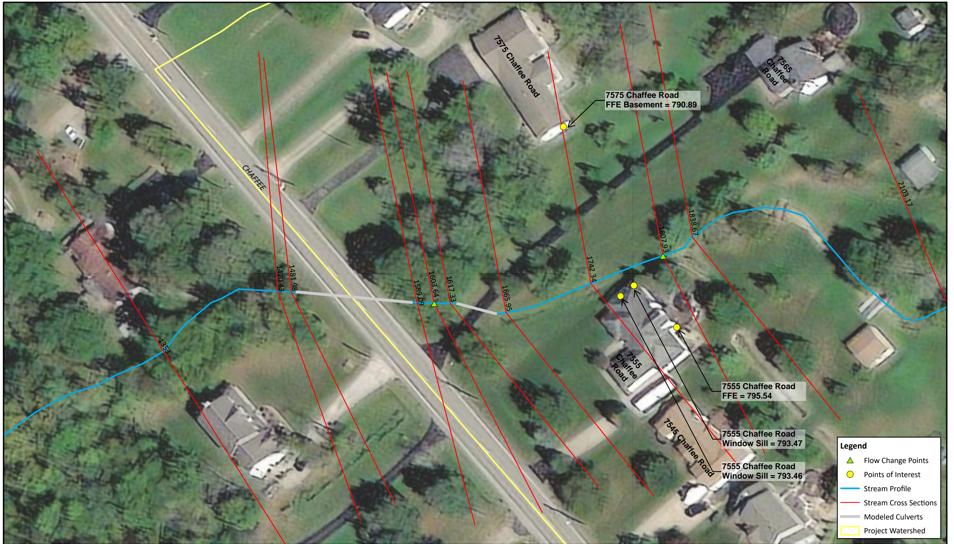
MAP 6: CHAFFEE ROAD PROJECT WATERSHED EXTENTS OF HYDRAULIC MODELING PROFILE FROM MEMO CHAFFEE ROAD WATERSHED STUDY MEMO SUMMIT COUNTY ENGINEER'S OFFICE
