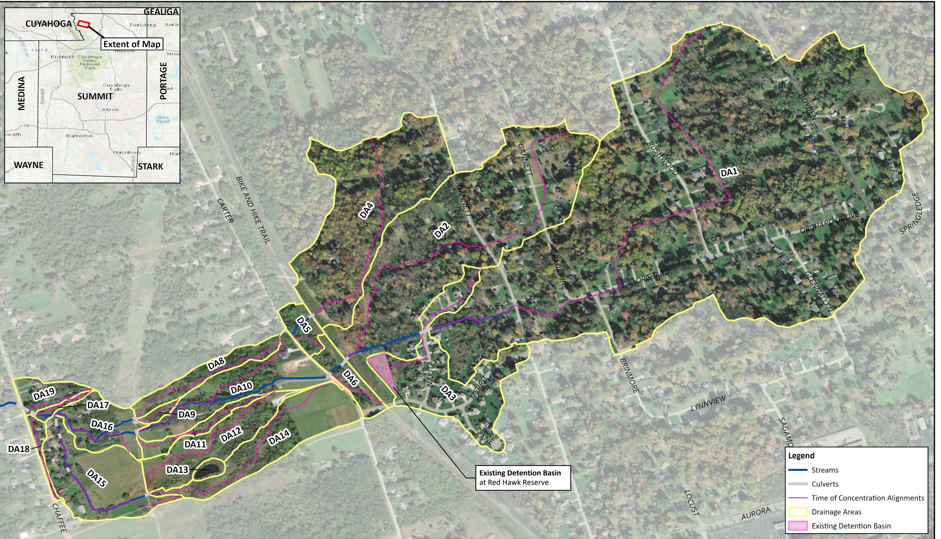
MAP 4: CHAFFEE ROAD PROJECT WATERSHED HYDROLOGIC MODELING DRAINAGE AREAS AND TIMES OF CONCENTRATION CHAFFEE ROAD WATERSHED STUDY MEMO SUMMIT COUNTY ENGINEER'S OFFICE
